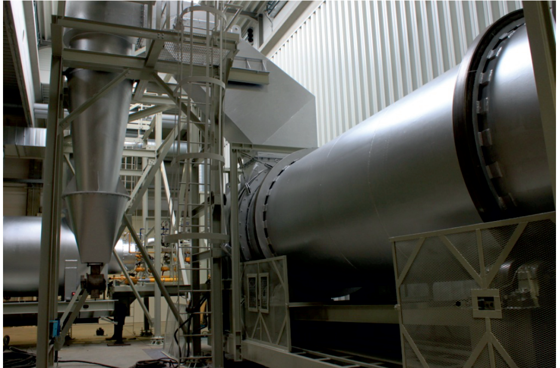
Figure: Rotary kiln for treatment metal containing bulk goods
